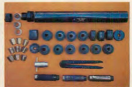
ABOVE: M30 suppressor disassembled: outer tube (top), followed by baffles, disassembly tools, and bushings to adapt the unit to different weapons. UPPER LEFT: Randy Franklin fires MAC-10, in caliber .45 ACP, equipped with Sionics suppressor and Dater's Superwipe. LEFT: Assortment of Dater's suppressors and weapons.
